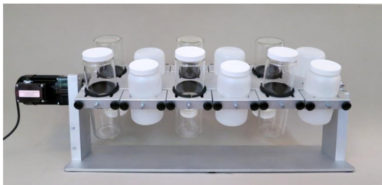
TCLP Rotary extractor used to spin samples for 18 hours
