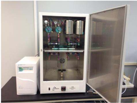
Canisters are cleaned for reuse in a computer controlled heated system. The system evacuates and refills the canisters and flow controllers with nitrogen multiple times to completely eliminate VOCs introduced during the previous sampling. System pressure and vacuum readings create consistent batch to batch cleaning.
