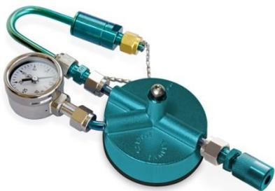
Our equipment provider, Entech Instruments, places a proprietary ceramic coating called **Silonite®** on the inside of sampling canisters and flow controllers to guarantee an inert surface, allowing the recovery of more compounds than any other air sampling device. Silonite® is a ceramic coating treatment developed by Entech to provide an ultra-smooth inert surface, surface which greatly reduces the potential for chemical adsorption.
